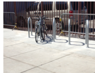
Inverted-U racks allow bicycles to to the rack in two places, providing stability and allowing the wheels and frame to be secured to the rack..
