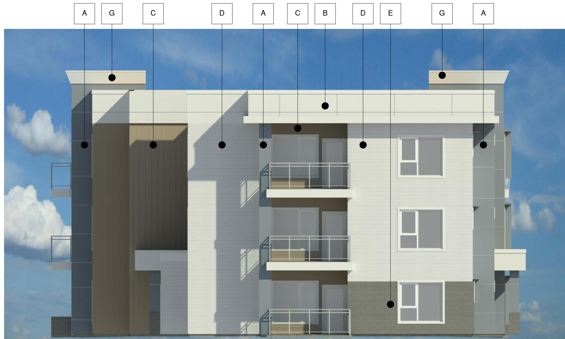
② BUILDING TYPE A LEFT ELEVATION - COLOR SCHEME 1
