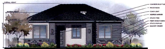
PLAN 2 PERIMETER UNITS FRONT ELEVATION ELEVATION B 1/8" = 1'-0"
