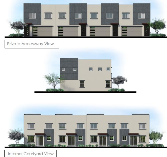
Figure J. Conceptual Elevation for 2 Garage Configuration. Top (Interior); Middle (Side); Bottom (Exterior)
