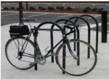
Inverted-U bicycle rack, where both ends of the “U” reach the ground.
