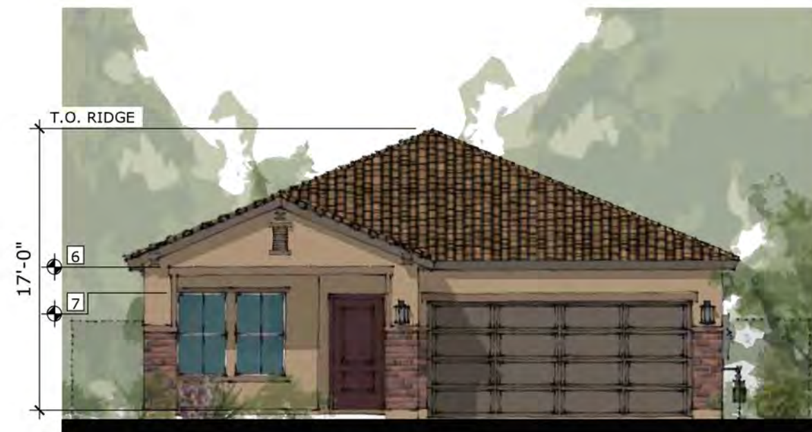
HACIENDA - FRONT ELEVATION SCALE: 1/8" = 1'-0"
