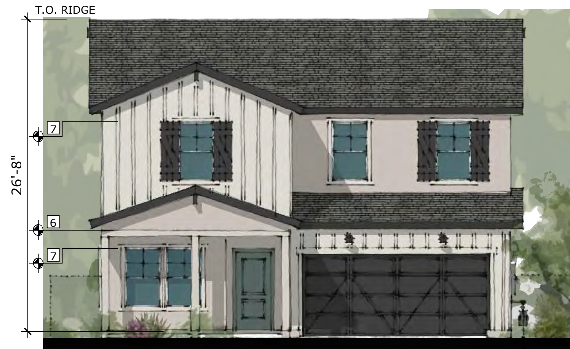
FARMHOUSE - FRONT ELEVATION SCALE: 1/8" = 1'-0"
