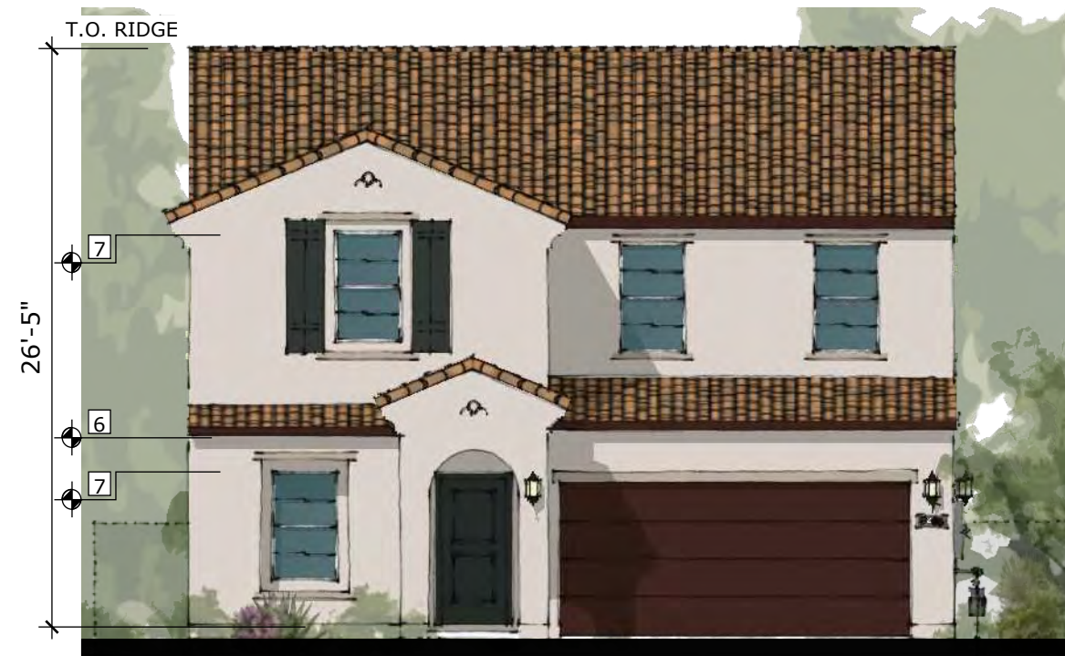
SPANISH - FRONT ELEVATION SCALE: 1/8" = 1'-0"
