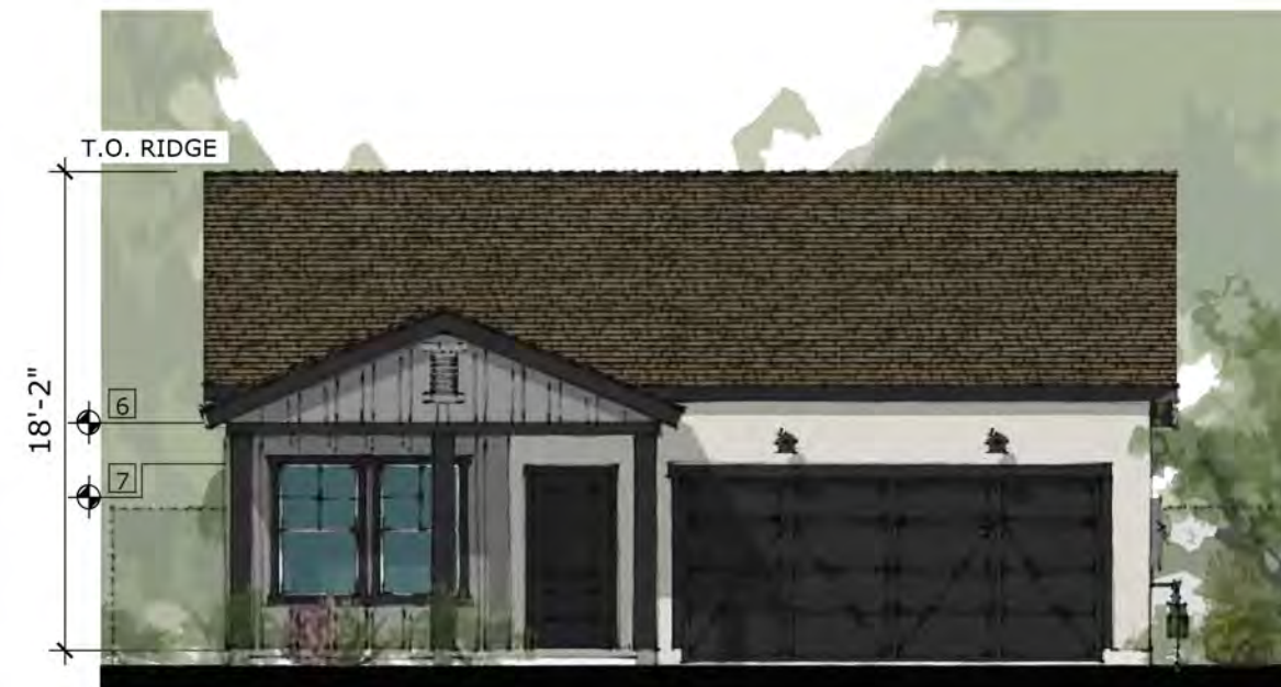
FARMHOUSE - FRONT ELEVATION SCALE: 1/8" = 1'-0"
