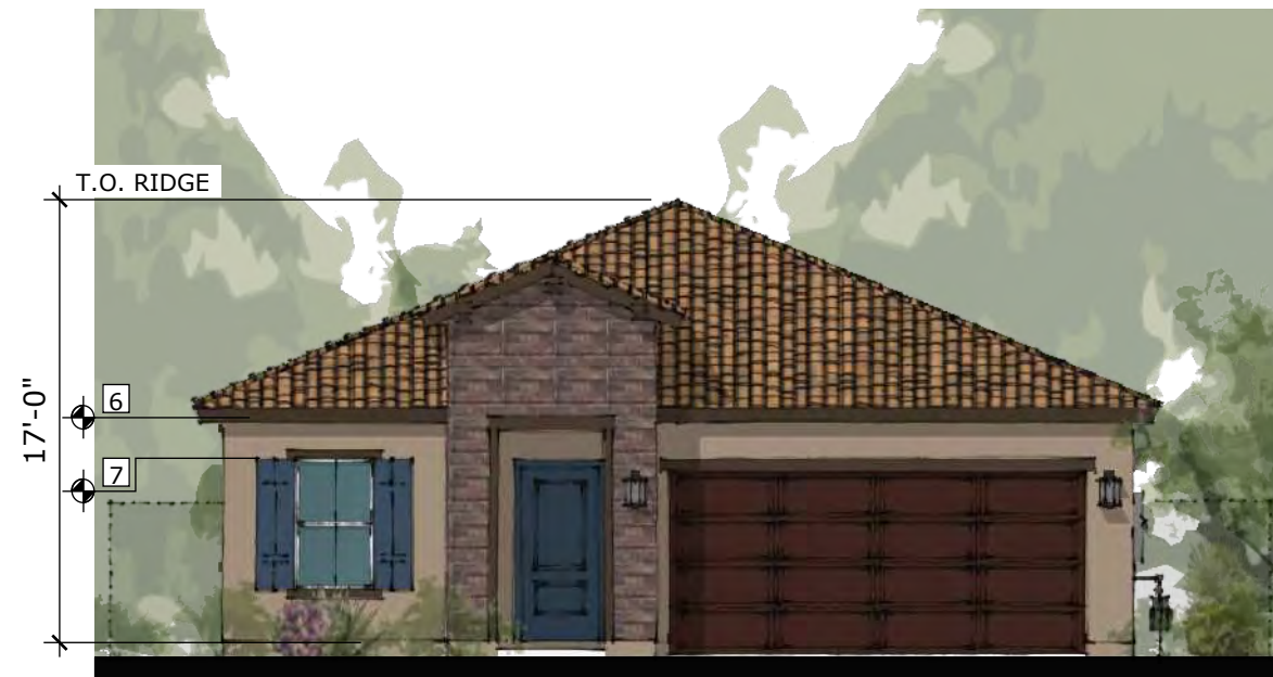
HACIENDA - FRONT ELEVATION SCALE: 1/8" = 1'-0"
