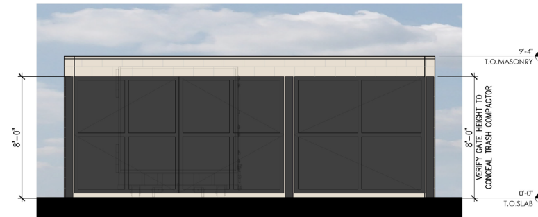
FRONT ELEVATION - COMPACTOR SCALE: 1/4" = 1'-0"
