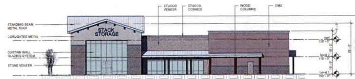
01 BUILDING 'A' NORTH ELEVATION 1/16" = 1'-0"
