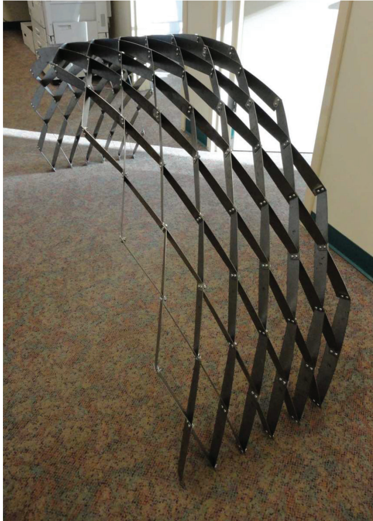
Figure 52 - Assembled Steel Lamella Arch.
