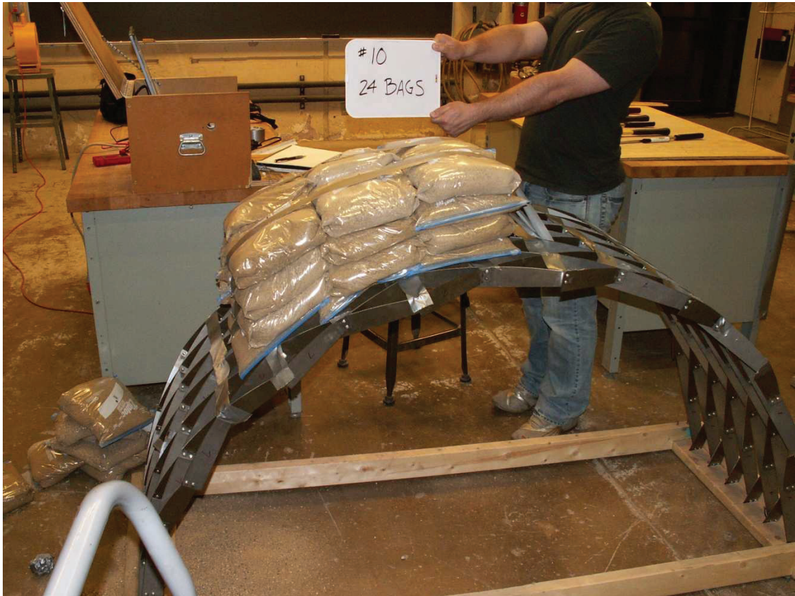
Figure 57 - Snow Drift Load Simulation.
