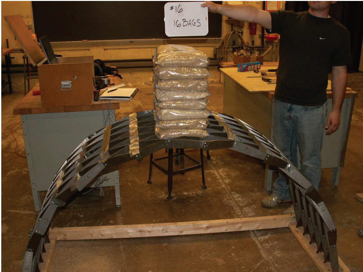
Figure 58 - Point Load Simulation.
