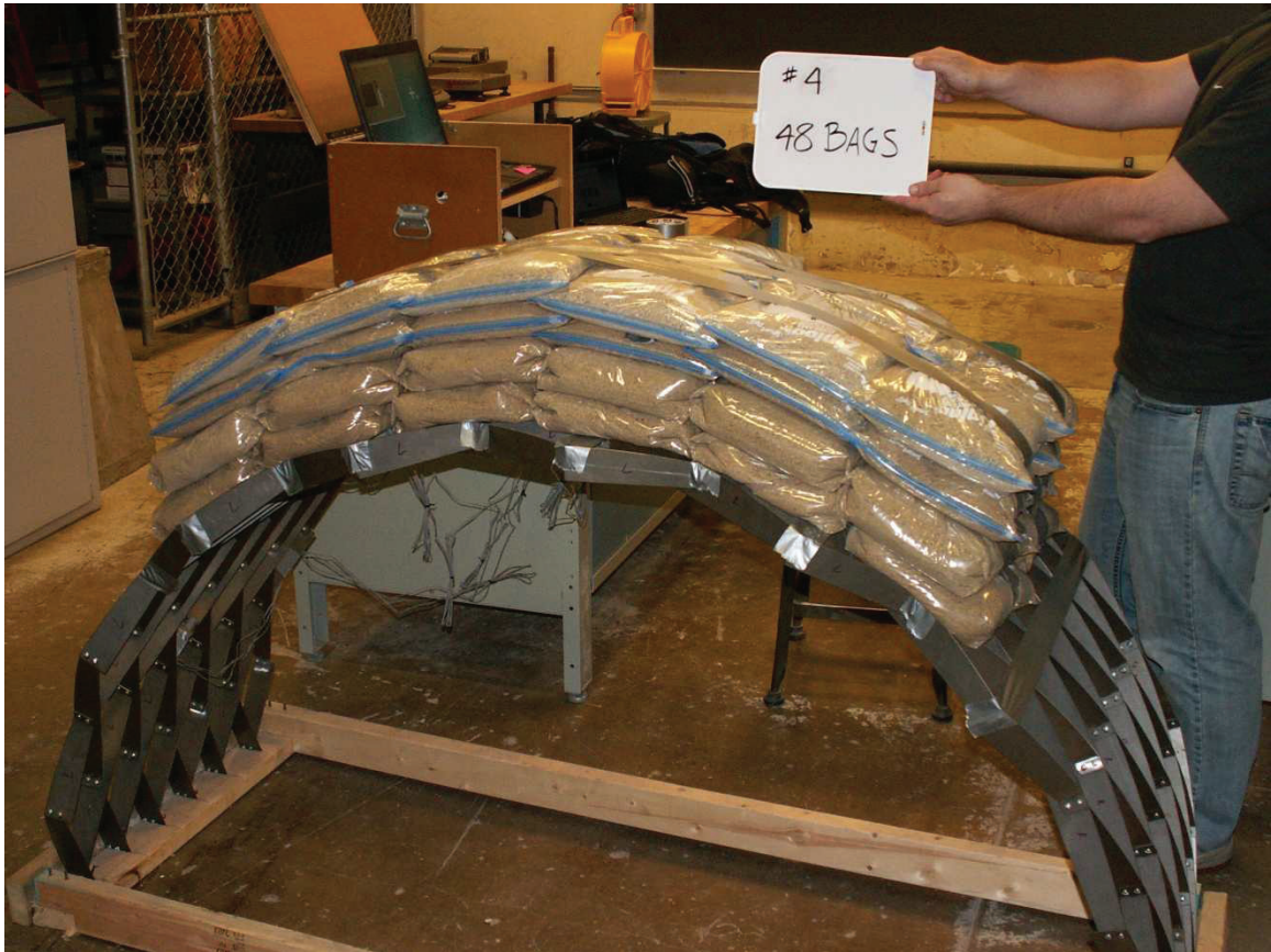
Figure 56 - Balanced Snow Load Simulation.
