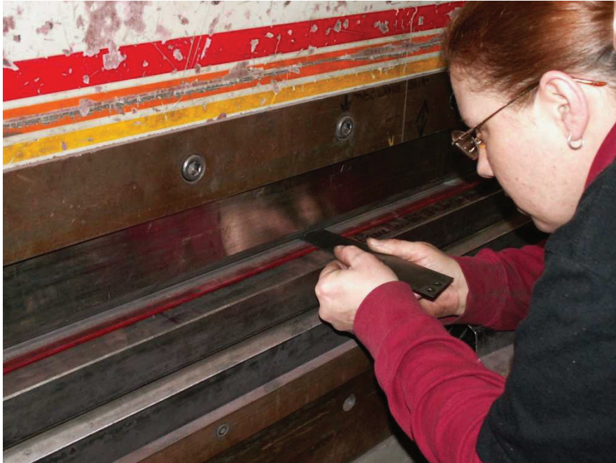
Figure 51 - Bending of Steel Lamellas.
