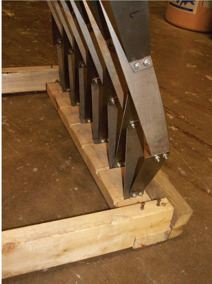
Figure 53 - Steel Model Bearing Plates.
