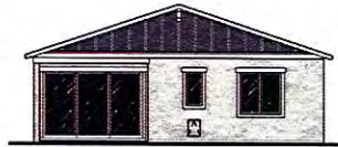
Rear Elevation Elevation B - Craftsman 1/8" = 1'-0"
