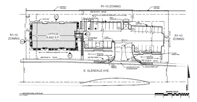
The eastern portion of the site consists of a parking lot containing 30 parking spaces. The trash receptacle is located in the center of the site, 25-feet from the rear property line, and aligned with the driveway.
