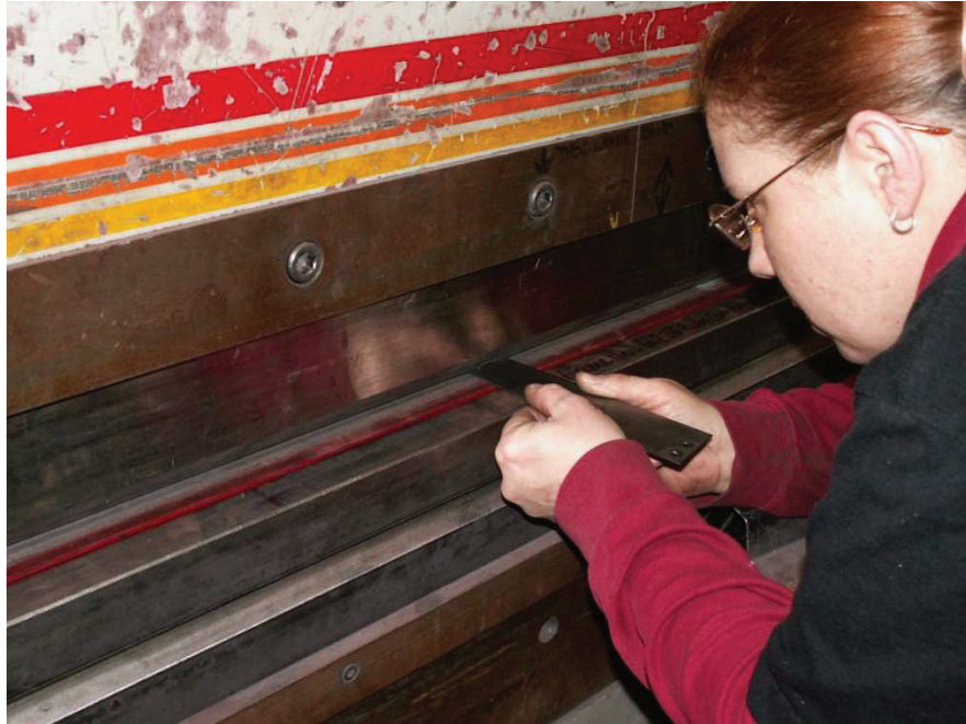
Figure 51 - Bending of Steel Lamellas.
