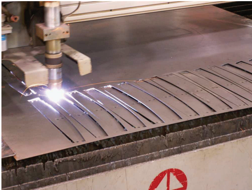
Figure 50 - Plasma Cutting of Steel Lamellas.
