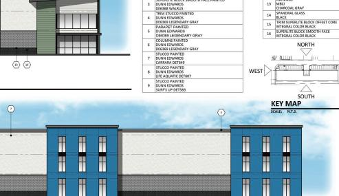
SOUTH ELEVATION SCALE: 3/32" = 1'-0"
