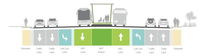
Lane configuration for center-running BRT along 35th Avenue at a signalized intersection where BRT stations are proposed.
