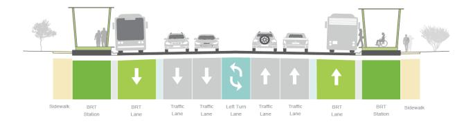
Lane configuration for side-running BRT along 35th Avenue at a signalized intersection where BRT stations are proposed.
