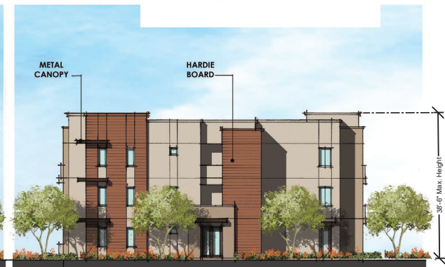
BUILDING 5- END ELEVATION
