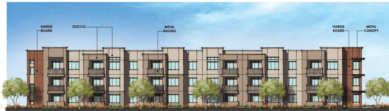
BUILDING 5- STREET SIDE ELEVATION
